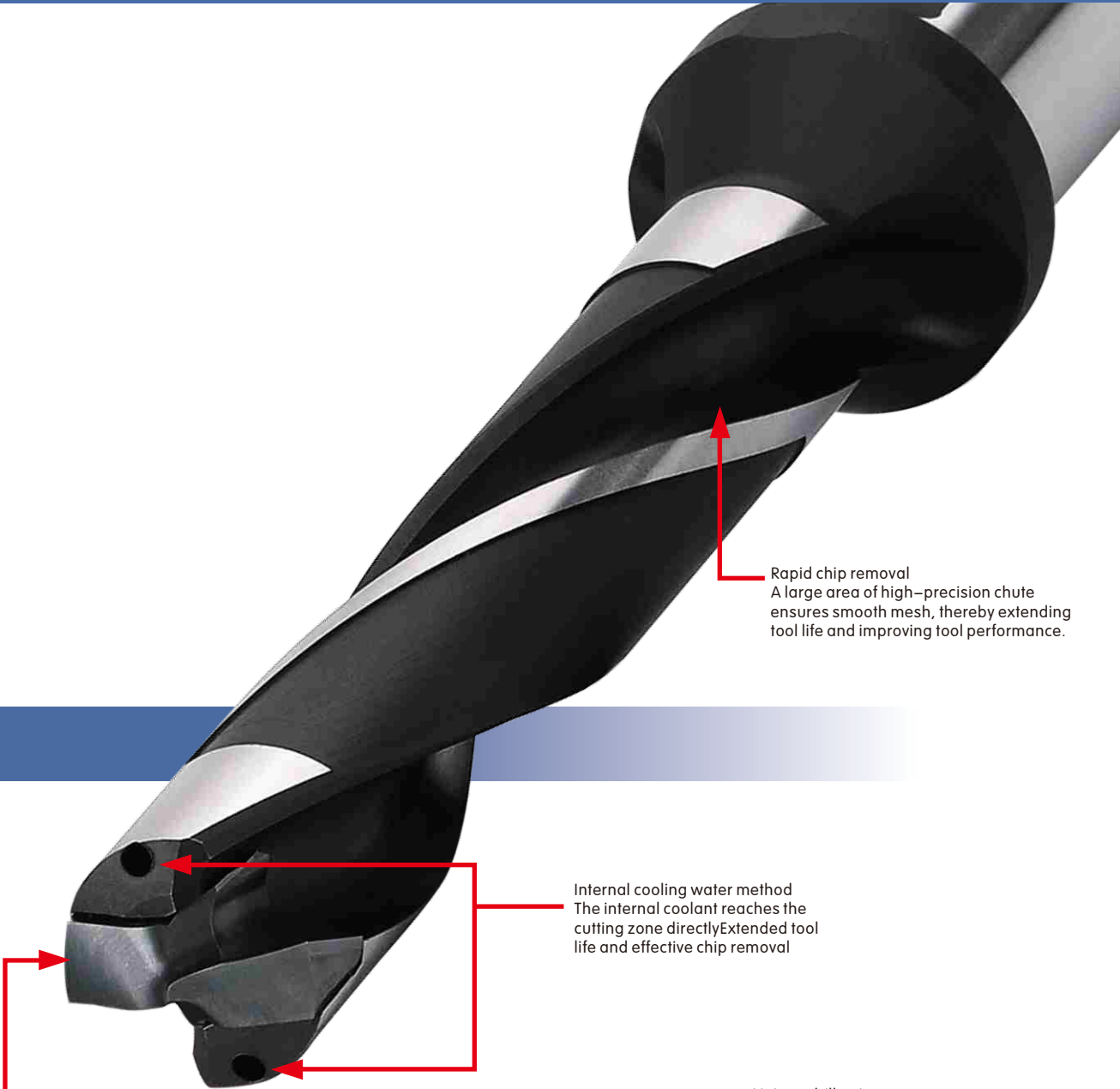
Unique drill point groove type Three special materials and self-centering tip design ensure excellent hole machining accuracy and optimized tool performance.
